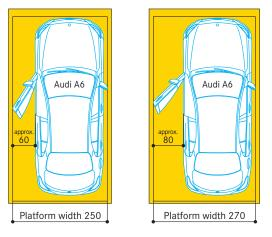
Depending on the vehicle model and the parking position of the vehicle on the platform, the space for opening the door varies. For comfortable conditions for getting in and out of the car, we recommend platform widths of at least 270 cm.
