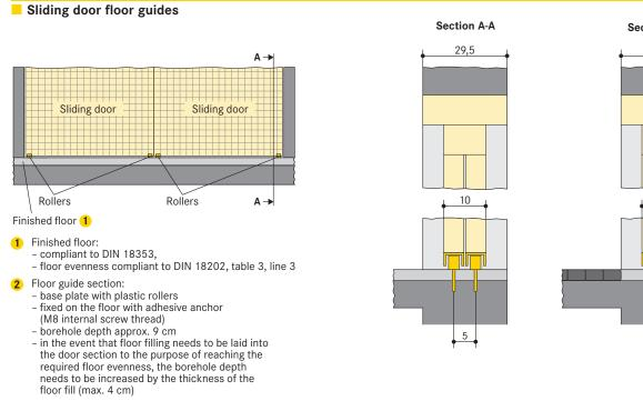
If the driving aisle is made of concrete blocks, asphalt etc., the concrete slab of the pit edge in the door area must be min. 29,5 cm wide 3
