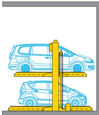
Before lowering the upper platform, the car on the middle level must also be driven off!
