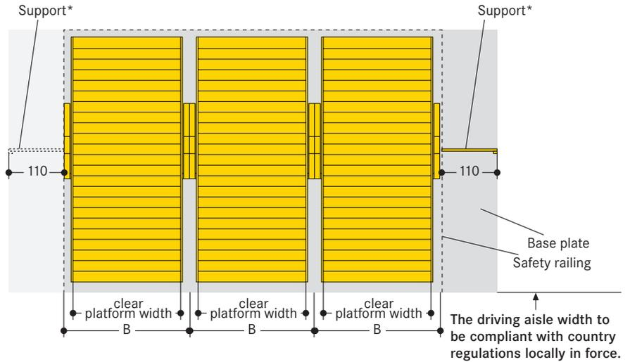
\* A one-sided support (either left or right) is sufficient. The base plate shall then be subject to both compressive and traction forces (see statics and construction requirements).
