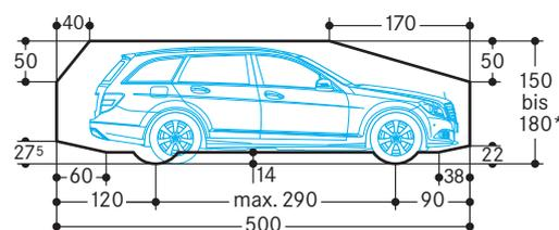
\* The total car height includes roof rail and antenna fixture must not exceed the mentioned max. height dimension.
