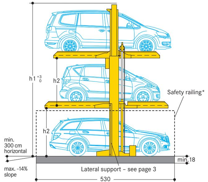
\* Rear and lateral site safety railing, compliant to the DIN EN ISO 13857 standard requirements, is to be supplied by the customer. The height of the safety railing is dependent on the distance from the moving parts.
