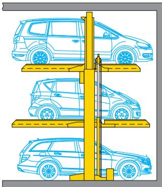
Before lowering the platforms, the car on the entrance level must be driven off!
