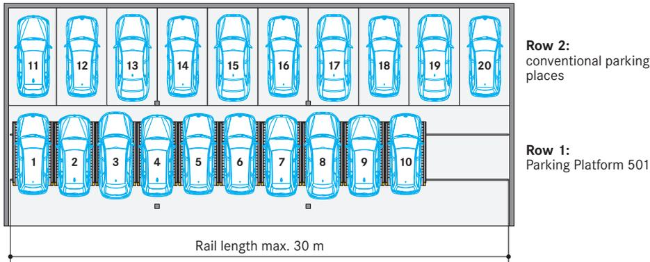
No light barriers are required for rails up to a length of 30 m.
