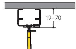
**Track and floor details (electric rail on the ceiling)**
