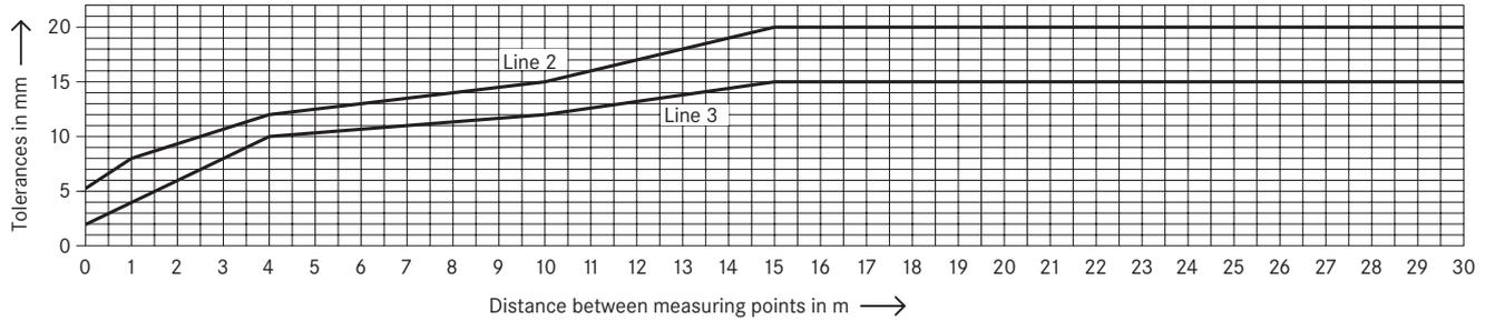
**Measuring points: finished floor (electric rail on the ceiling)**
