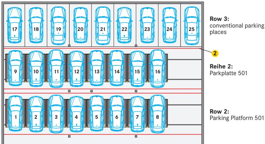
2 Light barriers must be provided for multi-row arrangements compliant to DIN EN 14010.
