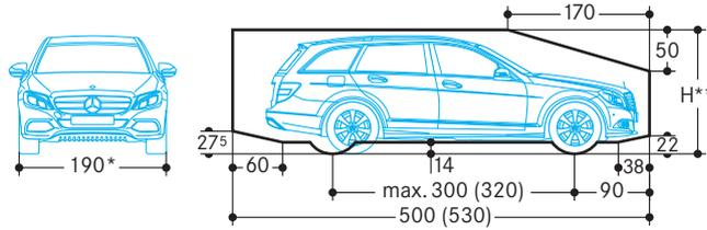
\* maximum lane + tyre width with platform width 217 cm
