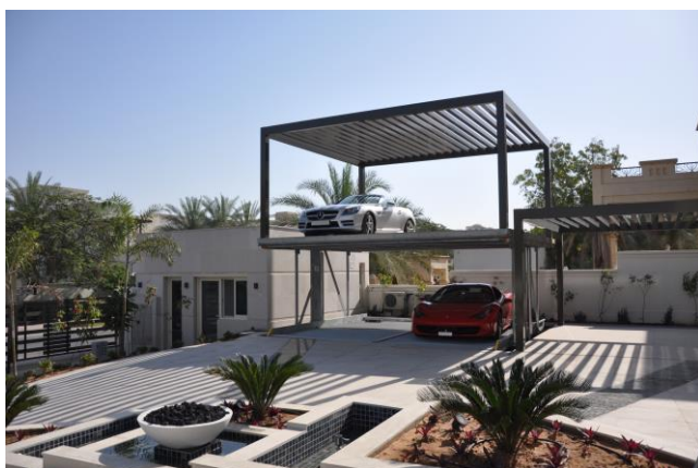
Image 1 and 2: The Parklift 461 D provides two underground parking spaces. A minor modification to the cover platform and adding the carport allows two additional parking spaces on the upper level.
